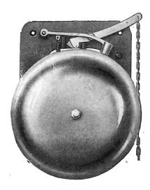
Best and loudest sounding Trip Gong made. One ring of Gong to each down pull of lever. May be fastened and will operate in any position. Black Japan; Hammer and Levers, Bronzed; Gong Shell, Nickel Plated
