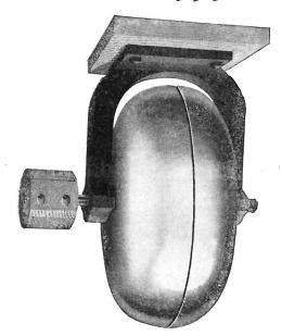
This gong is entirely automatic. It rings on any movement of crane or charging machine in any direction. Pulleys are not furnished with this gong but almost without exception they are arranged to furnish a speed of 80 Rev.
